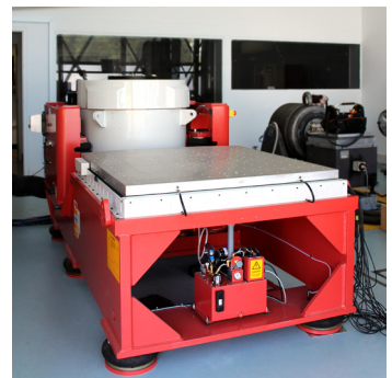
The LDS V8 Shaker Combo in Vipac's Port Melbourne Laboratory.
